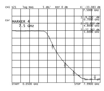
The curve illustrates the performance of the IMF2293 filter in a matched  $50\Omega$  alumina system.
