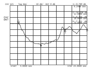
To the left is an example of a LPF that was designed for a specific customer application.
