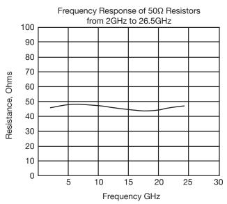
The response does not change appreciably at different resistance values. Similar response can be expected from other size resistors within the RCX PW Series and within the resistance range for the respective size.
