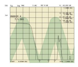
The curve illustrates the performance of the IMF2295 filter in a matched  $50\Omega$  alumina system.
